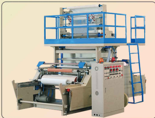
Type : T6 (Back-to-back auto. cut & auto. change reel winder, front cutter) 背對背全自動捲取機，前飛刀型式
